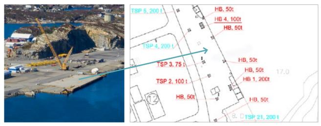
Quay 17 m depth:  $99 \times 43 \text{ m} = 4.200 \text{ m}^2$ . Load limitation 3 m from front quayside -  $80 \text{ kN/m}^2$  Quayheight MS L - 2.5 m
